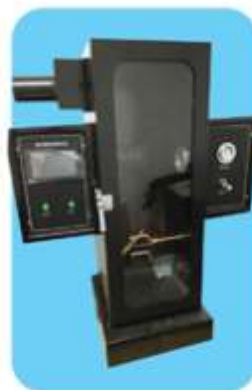
Smoke Density Test
